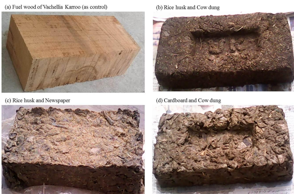
Figure 1. Fuel wood (as control) and samples of prepared bricks from organic wastes
