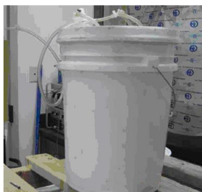
Figure 3. Leak test of reactor
