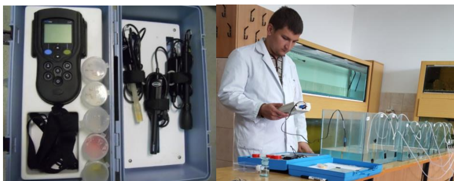
Figure 2. Portable analyzer, (Hach Products, Germany) used for measurements and research in aquariums
