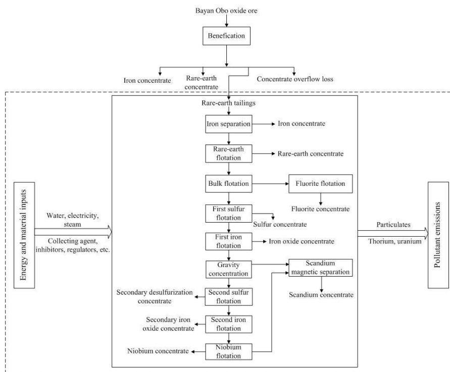
Figure 2. LCA system boundary of tailings integrated exploitation technology in Bayan Obo mine
