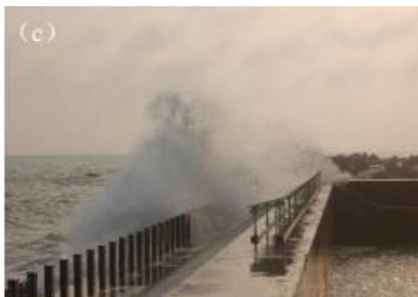
Figure 5. Marine environment test platform. (a) Atmospheric exposure test area; (b) offshore platform pilot zones; (c) splash platform test area
