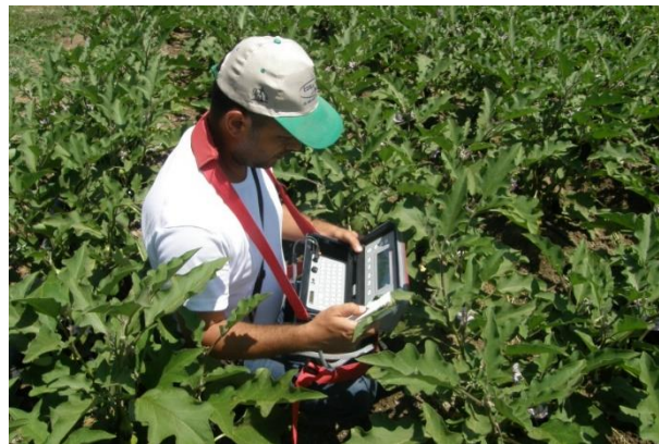
Figure 3. Measurement of stomatal resistance in eggplant with porometer
