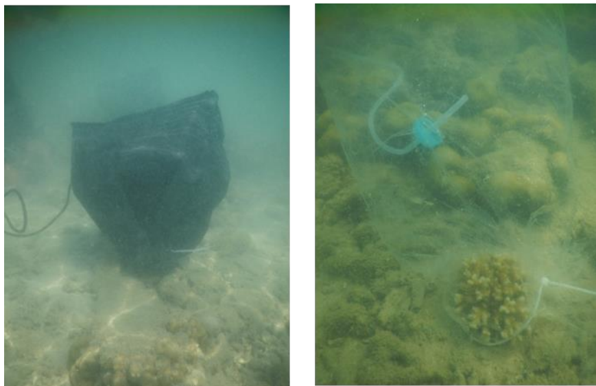
Figure 2. Dark (left) and light (right) benthic oxygen flux chamber ( n=3 )
