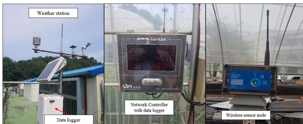
Figure 2. Images of local weather station, network controller with the data logger, wireless sensor nodes used in the experimental site
