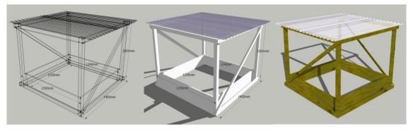
Figure 1. The dimensions of plots and climate control chambers
