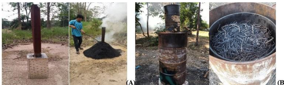
Figure 1. Biochar production used in this experiment: (A) rice husk biochar produced by farmer-traditional kilns and (B) rice straw biochar produced by biochar stoves
