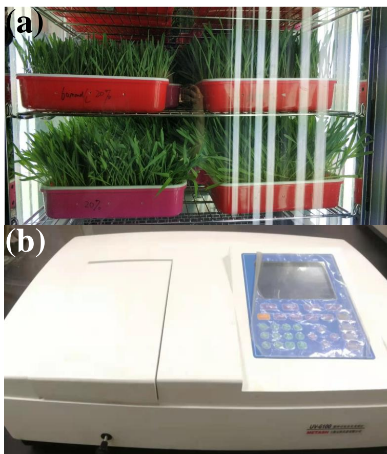
Figure 2. Photos of experimental culture and equipment. (a): 9-day barley seedlings in light incubator. (b): UV-6100 UV-visible spectrophotometer (Metash Co. Ltd)
