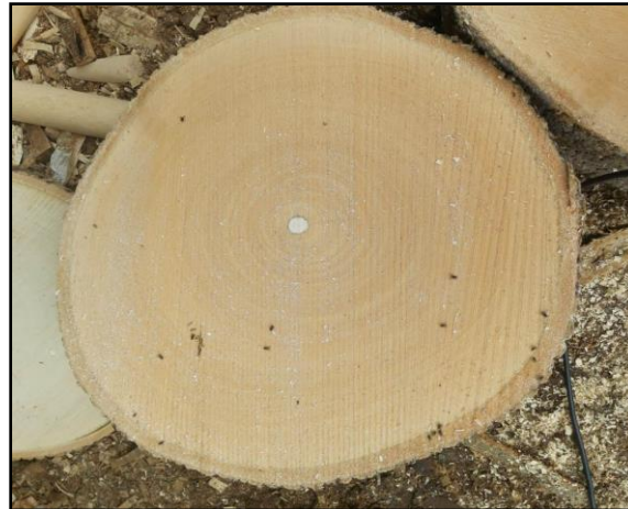
Figure 2. Round disc was taken from the tree's breast height (1.37 m) for the cutting out samples of the radial positions
