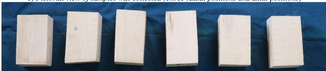
d) 2x2x2 cm 3 samples were taken out from round disk
