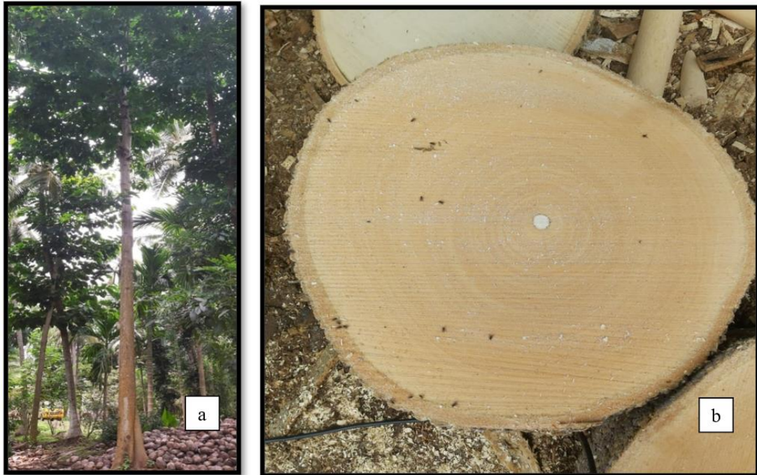
a) Pterygota alata tree grown in farm condition b) Round disc collected from three different axial positions
