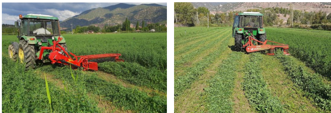
Figure 3. Disc mower with conditioner (left) and drum mowers (right) used in the study
