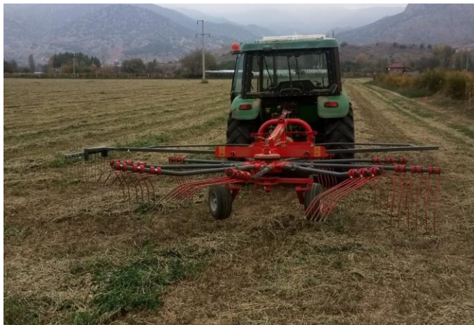
Figure 4. Nine-armed rotary rake
