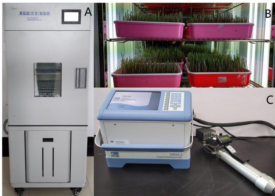
Figure 1. Photos of experimental culture and equipment. A: BPHJ-120A a test chamber with alternating high and low temperature (Shanghai Yiheng Scientific Instruments Co., Ltd). B: 7-day rye seedlings in light incubator. C: CIRAS-3 photosynthesis measurement instrument (Hansha Scientific Instruments Co., Ltd)
