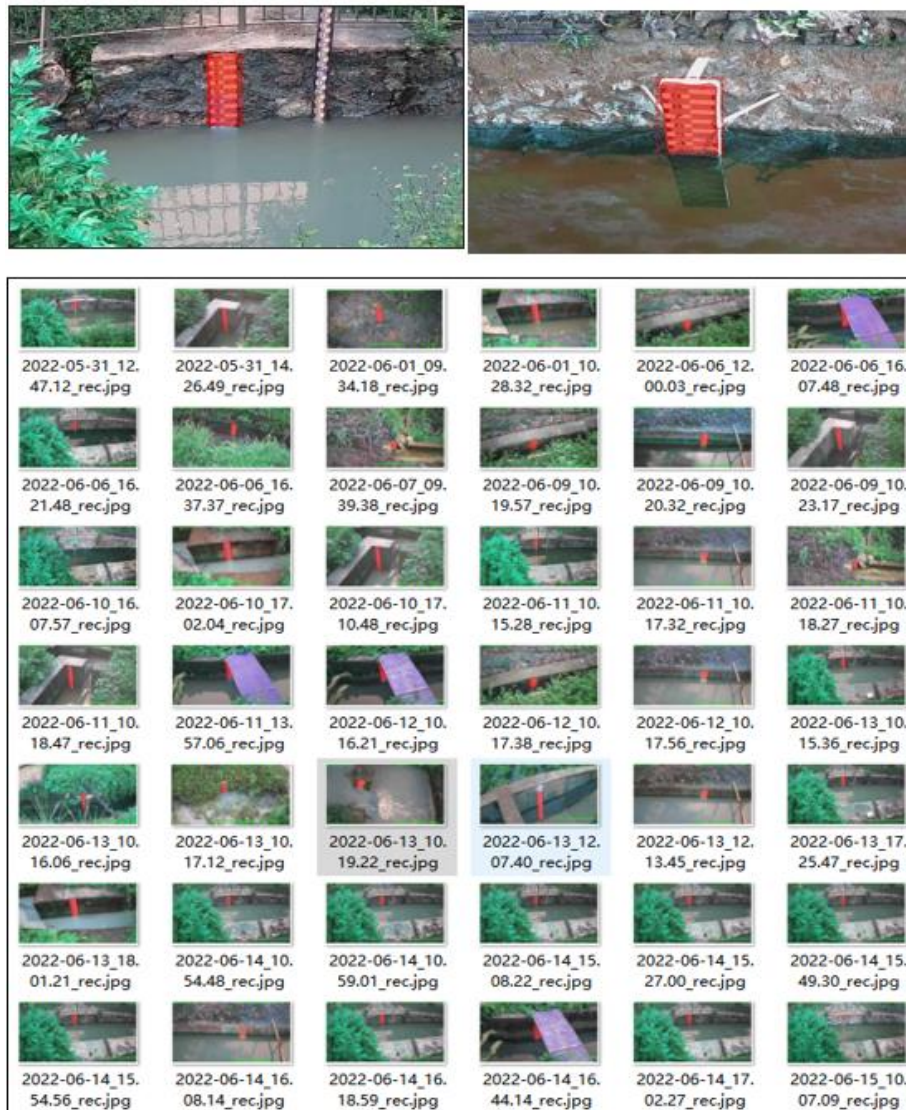
Figure 5. The effect of water gauge target recognition and edge extraction
