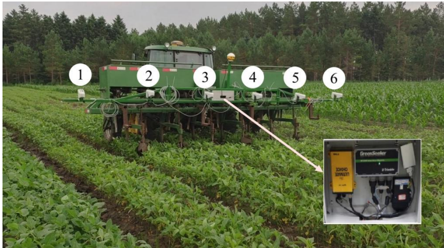
Figure 2. Soybean NDVI data acquisition system (the number in the figure represents the position of the sensor)
