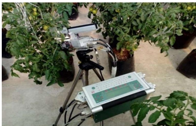
Figure 2. Reading of gas exchange variables and chlorophyll fluorescence efficiency in mycorrhized tomato plants through a portable system for photosynthesis measurements LI-6400XT (Li-Cor. Inc.)
