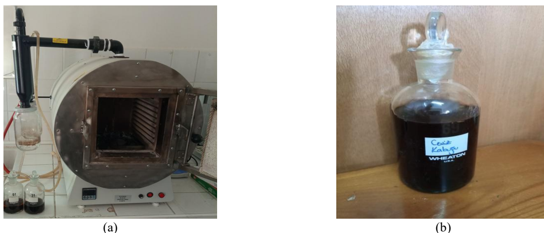
Figure 1. (a) Double condensing PID controlled biomass pyrolysis system. (b) Pyrolysis liquid (PL)
